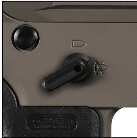
Safety selector in “fire” position
